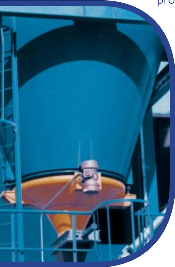
The Bin Activator is extensively used to ensure the product is discharged efficiently and effectively in a controlled manner from a silo or hopper.
