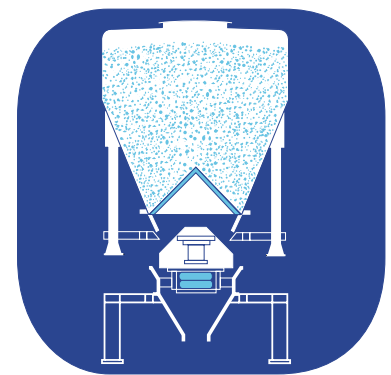
1. Bin lowered onto discharge station.
