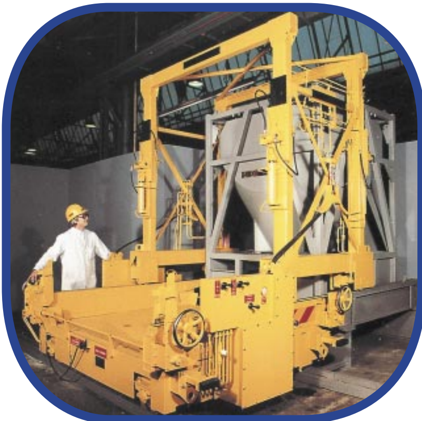
Special IBCs produced for offshore oil rigs to handle drilling 'mud'. Rail mounted to save headroom.
