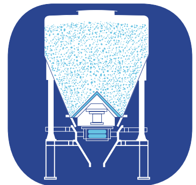
2. Bin sealed in position ready to discharge.
